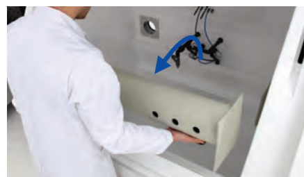
1. The air system collection tube is easily removed.
